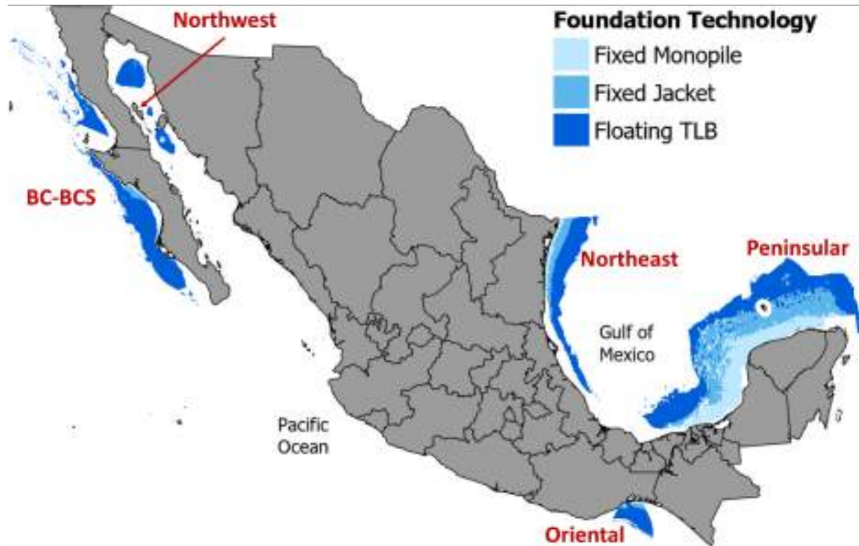
Figure 6.5: Foundation Type and Ocean Suitability by Depth for the Five Designated Zones of Offshore Wind Energy Deployment.
